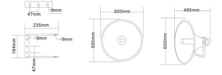
**Description:** All aluminum alloy structure, wide frequency domain waterproof horn, large power, strong sound penetration, wide coverage, suitable for square, railway station, etc.
