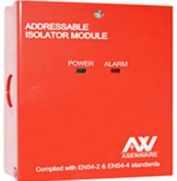
other parts of the system can work normally. Meanwhile, the isolator module also can help find out the faulty bus part. After the faulty part is repaired, the isolator module can back to work by itself, including the isolated part into the system again.
